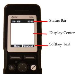
The display is divided in three parts: **Status bar**, **Display center** and **Softkey Text** (see figure above).
